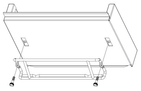
Attach the new hanger, as shown below, with the provided screws.
